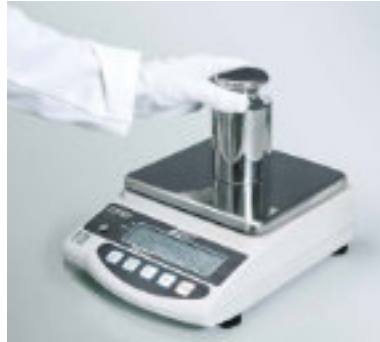
Initial calibration and recalibration of balance at the KERN factory
