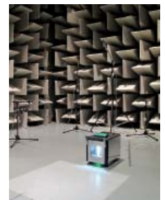
ISO 3744 acoustic test
